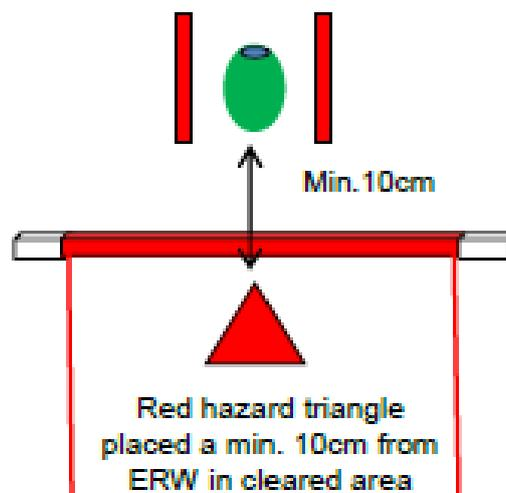
Figure 5: Example - Marking a located ERW or other hazardous object
